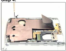
Lift off the back cover. Remove ONLY the Phillips screw shown in the picture above, then fold back the protective copper foil (taking care not to tear or damage it) so that the battery can be reached. Set the screw aside for reassembly.
